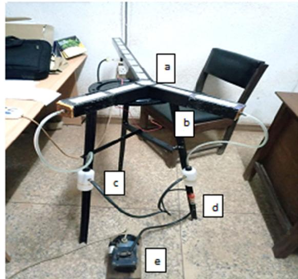
**Figure 1: Set up showing the connection to the 2-way olfactometer: a, 2-way olfactometer; b, metal stand; c, test odour/control container; d, air filter; e, air pump**
